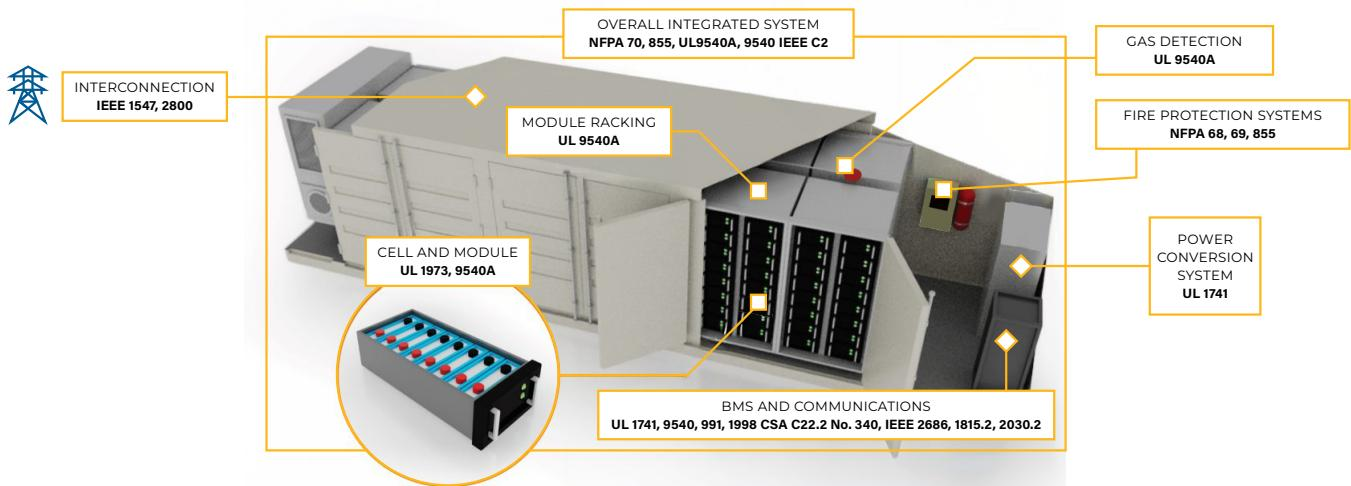
*This image is adapted from PNNL. While it shows a walk-in area that would result in it being treated as an indoor installation under NFPA 855, the intent is to show C+S applicability for outdoor installations only.*
